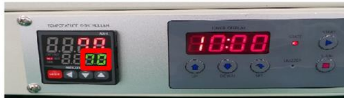
Put the device in to HOT PLATE.(70°C/10mins)
