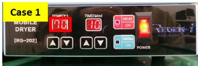
Put the device into Mobile Dryer.(70°C/10mins)
